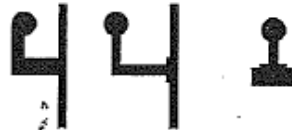
GRIPPABLE HANDRAIL DESIGNS: Grippable Area = 1 1/4" to 2" cross section
